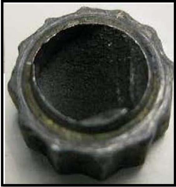
Figure 3 OMEGA Head Bolt and Shank Failures (3)
