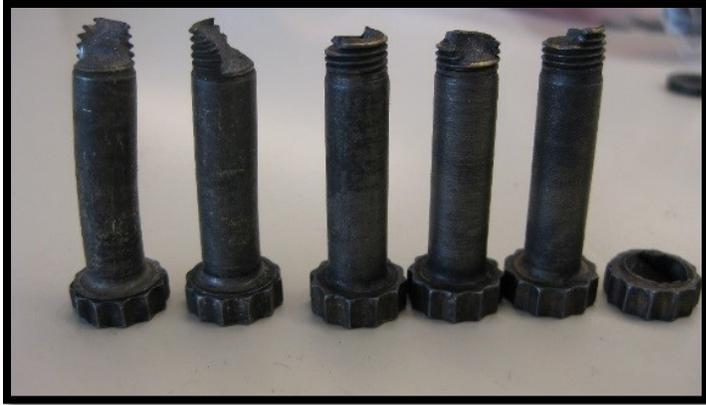
Figure 1 OMEGA Head Bolt and Shank Failures (1)
