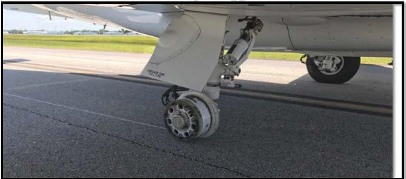
Figure 4 Beech Jet 400A, Service Wheel Separation
